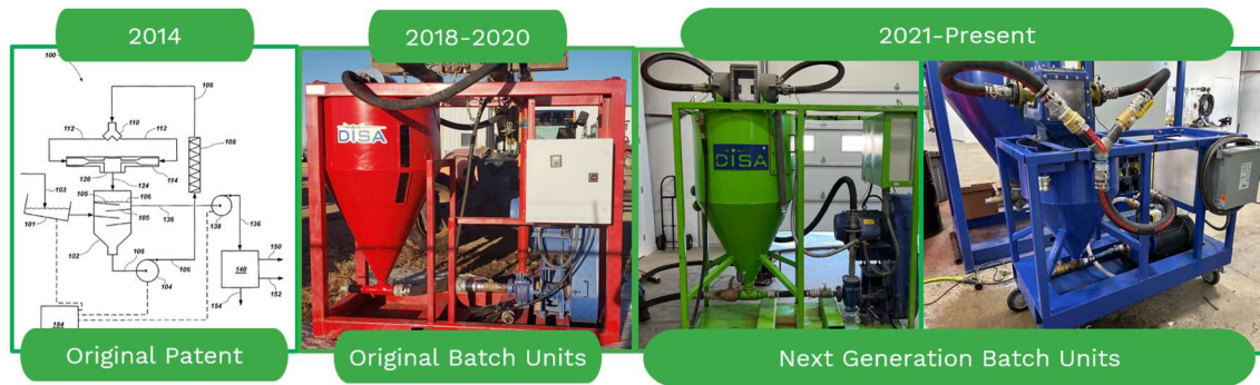
Figure 3: Evolution of the HPSA batch unit from the original patent to first prototype, to Lab and Lab Bench Scale units.
